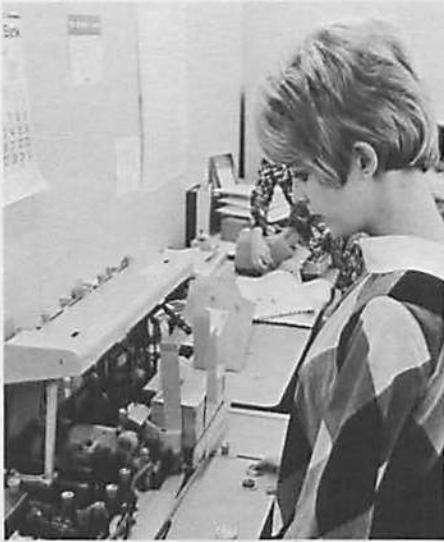
Nancy Anders operates new machine that stuffs and seals pay check envelopes.
