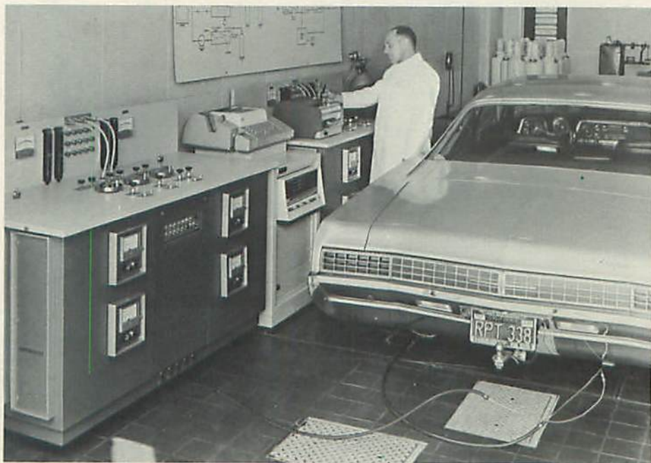
Beckman Vehicle Analysis System uses PDP-8/S in automobile exhaust test. Photo courtesy of Beckman Instruments, Inc.
