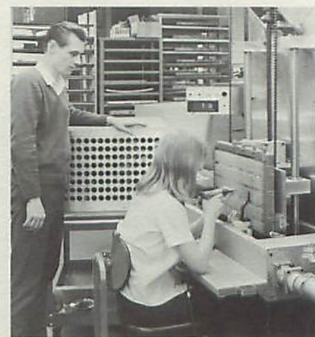
Rick Mead looks on as Marion Walford wires another PDP-8/I logic frame. The wire wrap machine is one of eleven at Carleton Place, all of which are numerically controlled by a PDP-8.
