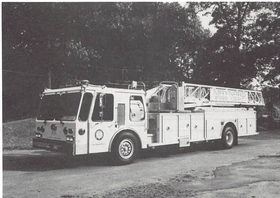
LADDER 1 - 1986 EMERGENCY ONE WITH 100 FT. AERIAL LADDER.
