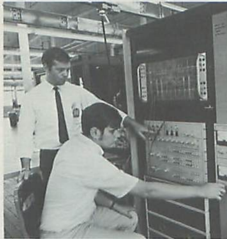
Phil Despo (l.) and Ernie Strange demonstrate the use of the PDP-15 Memory Exerciser.
