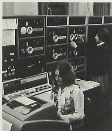
Sheila Ford takes her turn on the PDP-10 Teletype, while Margaret Ewings changes DEctapes.
