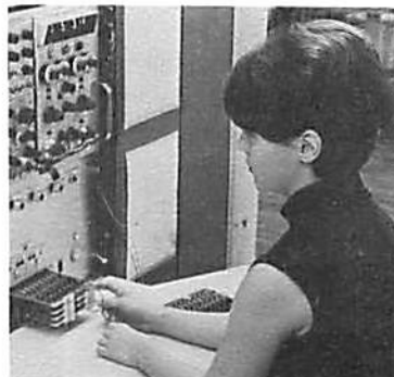
Barbara Manard checks a module using Module Testing's PDP-4 and automatic tester.
