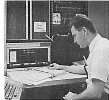
George Turner checks data on the PDP-8 used to operate the automatic wirewrap machine.
