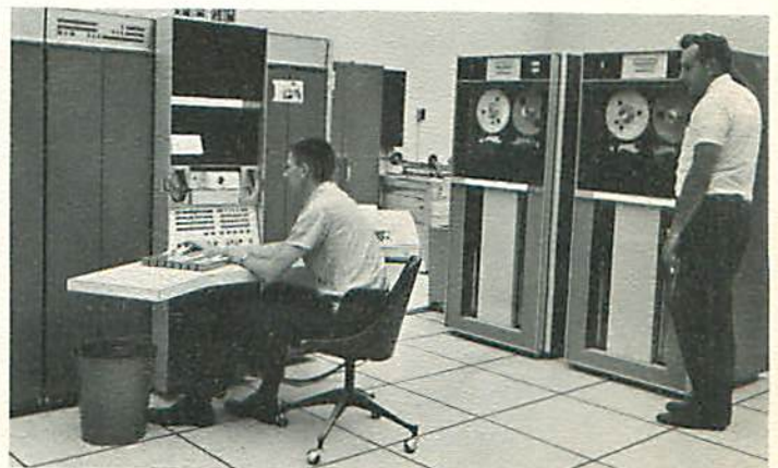
At LASA Data Center -- A PDP-7 and two tape units are shown in operation at the Billings, Montana, LASA Data Center, recording and processing information from 525 seismometers scattered over 10,000 square miles.
