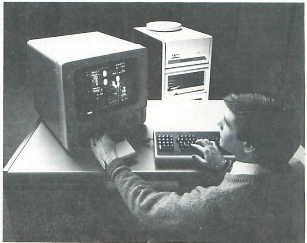
Digital's new VAX-11/730 32-bit minicomputer supports interactive graphics workstations using Digital's VS11 terminal for engineering design, as well as educational and commercial applications with up to 24 concurrent users.
