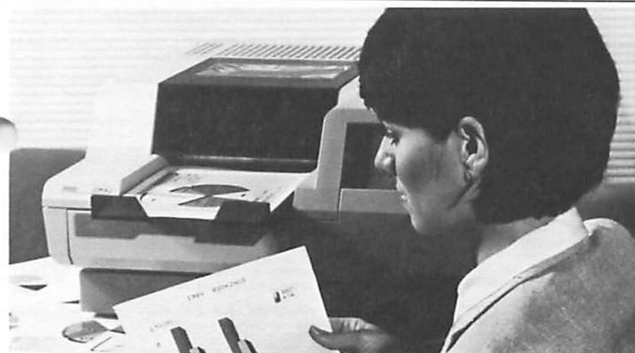
The LCPO1 ink-jet color graphics printer contains Digital's J-11 microprocessor and page-buffer memory that take the burden of graphics processing operation off the host computer system.
