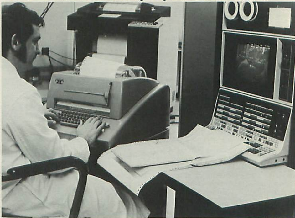
A technologist enters doctors' requests for laboratory analyses on the Teletype of DEC's new CLINICAL LAB-12 advanced clinical laboratory computer system. The system monitors and processes data from laboratory instruments, which analyze blood, urine, and other body fluids.
