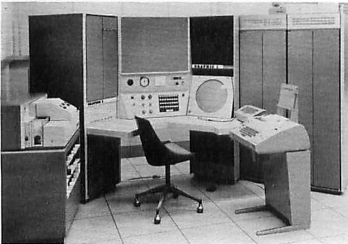
View of the Bell System—Bell Telephone Laboratories sends this photo of their PDP-5/340 system in the Signal and Information Processing Research Department, Murray Hill, New Jersey. The PDP-5 computer and Type 340 Incremental CRT Display form the heart of a new interaction system which will be used both to enter and to receive graphical data in the Laboratories' Computing Center.
