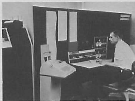
PDP-9 computer is master control unit of a highly accurate computerized launch vehicle/spacecraft guidance, navigation, and control simulation system.
