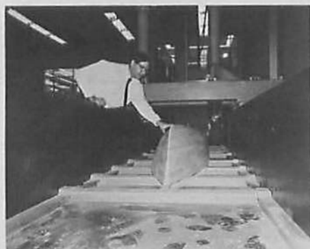
Dr. D. Gospodnetic checks keel of boat model which has been milled from a large block of wood using a PDP-8/I computer.
