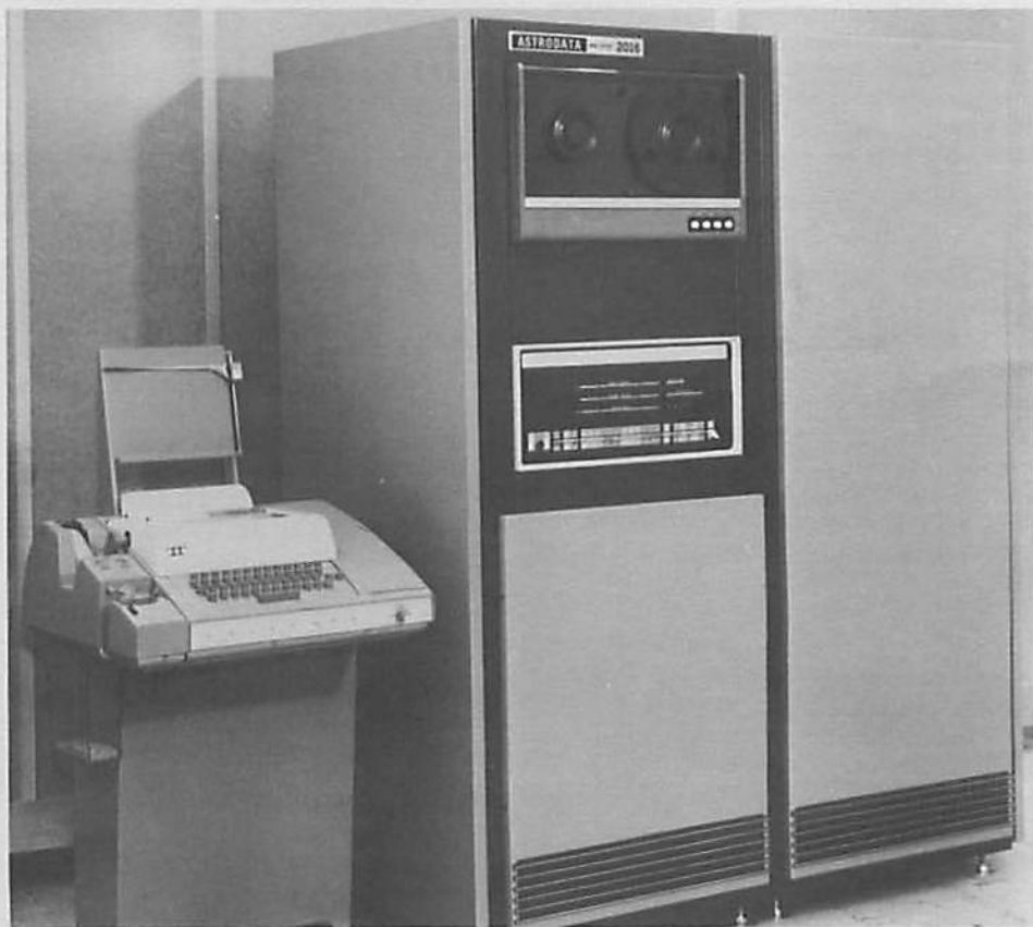
Latest data acquisition system from Astrodata, Inc. of Anaheim, California is an analog and digital system using DEC's PDP-8/L computer as the central control element.
