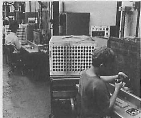
Wire wrap operators at Carleton Place produce logic panels for several DEC computer lines, all under the control of a PDP-8 computer.
