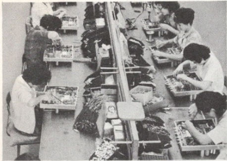
Unique assembly line techniques. After every 3 assembly line steps, there is an "in process" inspector who checks for "cold," or unsoldered joints, lead dress and short circuits. Here we see one of these "in process" inspectors giving one of the 50 such checks each Scott component receives before being shipped.
