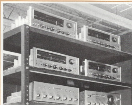
Long component life is assured by rugged "life test" rack. Here production units are subjected to "on-off" cycles and voltages far in excess of those encountered in home use. Three months on this rack is equal to 10 years of normal use.
